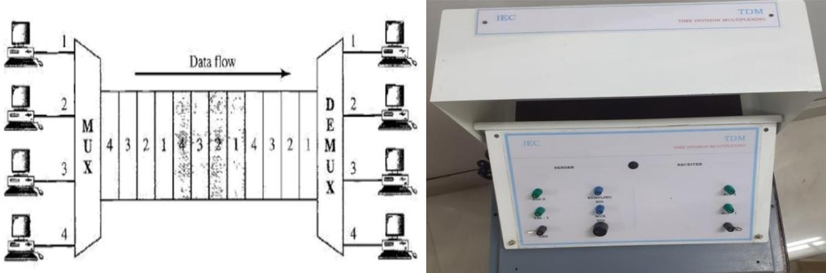
Multiplexing is used to combine multiple communication links into a single stream.
