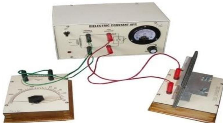
Dielectric Constant Apparatus is used to measure dielectric constant of different solids such as Bakelite, Teflon etc and liquids such as distilled water, transformer oil etc.
