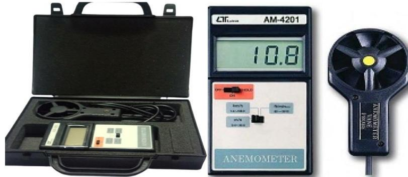
Anemometer is a device used for measuring wind speed. When the anemometer faces the wind, concave surfaces of the cup create more resistance than its convex surfaces and hence an unbalanced moment is produced which causes rotational motion with respect to its centre axis. Under steady flow condition, the rotational speed of the anemometer is directly related to the wind speed.
