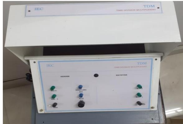
Multiplexing is used to combine multiple communication links into a single stream.
