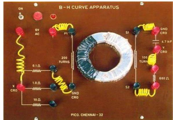
B-H Curves and Hysteresis Loops are valuable tools for comparing the characteristics and behaviour of different magnetic materials, in order to select them for an appropriate applications.
