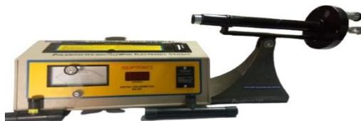
Polarimeter is used to determine the specific rotation and optical rotation of products such as amino acids, antibiotics, dextrose, carbohydrate, vitamins, steroids, sugars, serums, etc.
