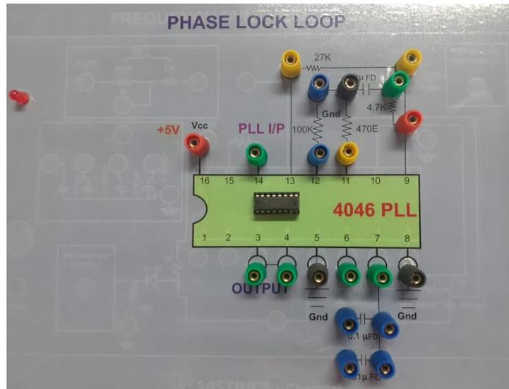
The phase locked loop is used in radio frequency or wireless applications.
