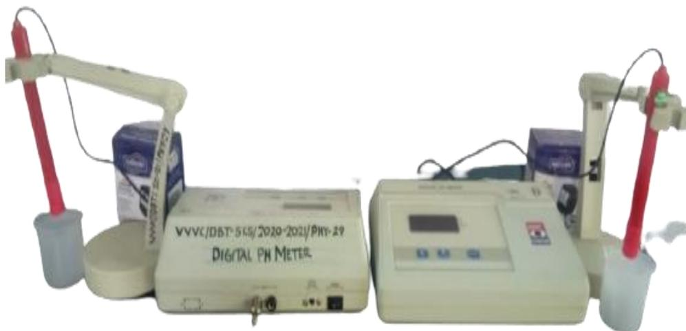
A digital potential of hydrogen (pH) meter is an electronic gadget used to measure accurately measure and record the pH value of liquids. Measuring pH allows one to determine the acidity or alkalinity of a substance in a liquid state.
