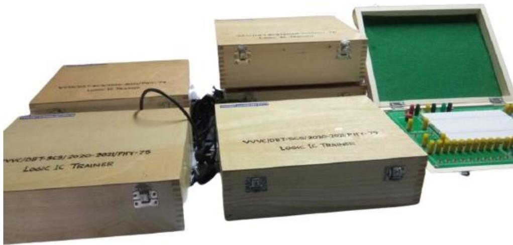
1. Digital IC trainer kit is used to study the operation of digital Logic ICs TTL, CMOS, AND, OR, NOT, NAND, NOR, XOR Gates, Flip-Flops, Counters, Shift Register, Multiplexer and De-Multiplexer, Encoder, Decoder and ALU.
